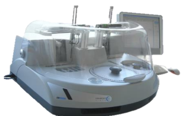
Fig.1 TG was determined fully automated under standardized conditions on the coagulation analyzer Ceveron® α TGA with Ceveron® TGA RB assay kit.
